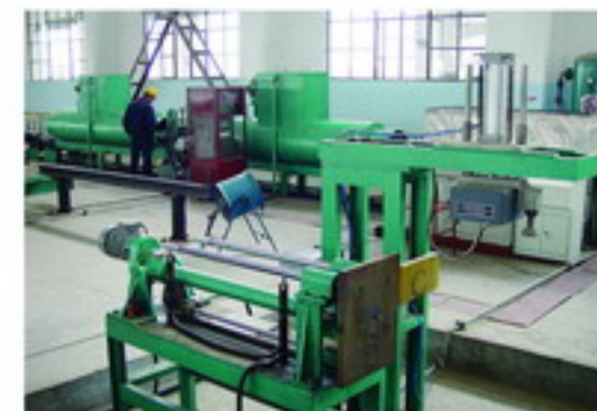
套管称重测长、打标、喷标设备 Weighing, length measuring and marking equipments for casing pipe
