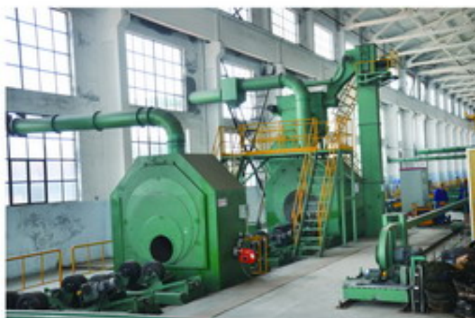
3PE (3PP) 防腐钢管外壁抛丸清理机 Φ32mm-Φ1820mm External Shot Blasting Cleaning Machine For 3PE (3PP) Coated Steel Pipes O.D.32mm-O.D.1820mm
