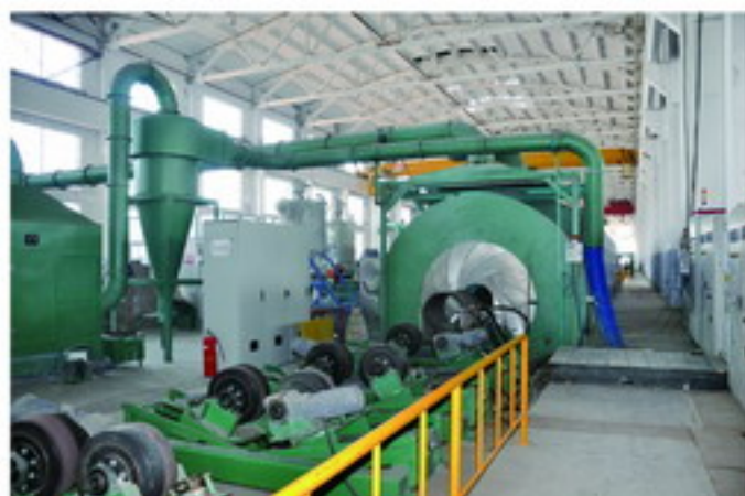
3PE (3PP) 防腐钢管生产线 Φ32mm-Φ1820mm 3PE (3PP) Coated Steel Pipes Production Line O.D.32mm-O.D.1820mm
