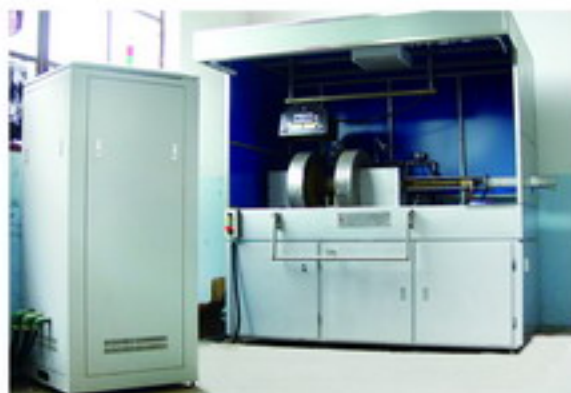
SMT/CZW-4000 磁粉探伤机 SMT/CZW-4000 Magnetic Particle Testing Machine
