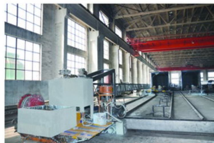
环氧防腐钢管液体环氧涂料内喷涂机 Φ508mm-Φ3620mm Liquid Epoxy Internal Spraying Machine For Epoxy Coated Steel Pipes O.D.508mm-O.D.3620mm
