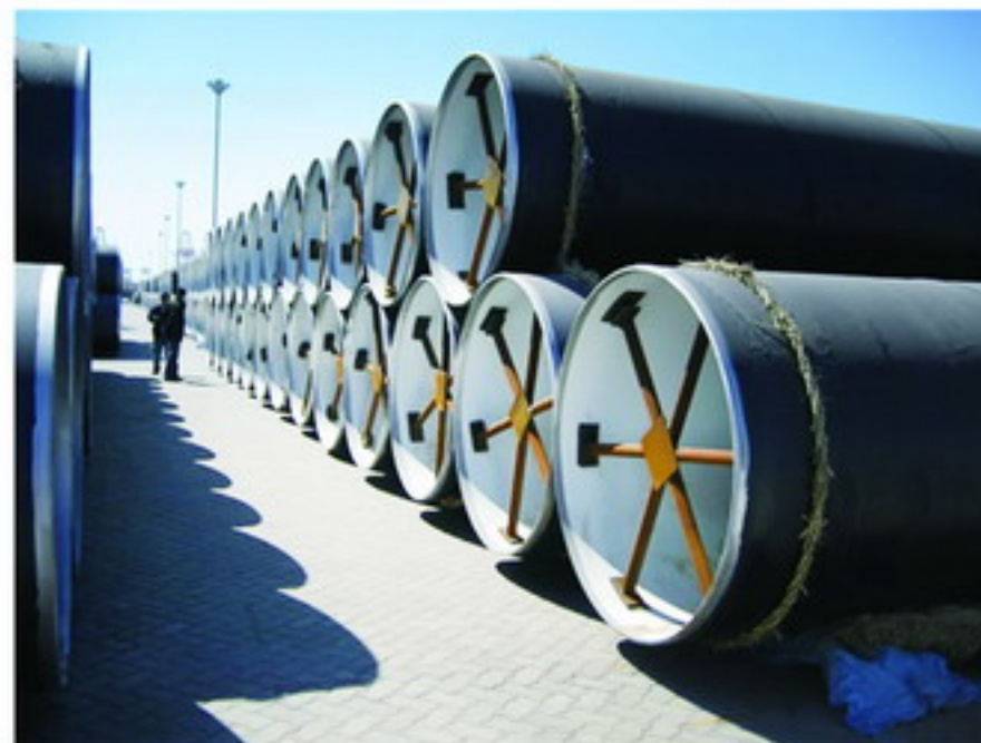
环氧煤沥青防腐钢管 三布五油 Epoxy coal bitumen anticorrosion steel pipe (with three layers cloth and five layers oil)
