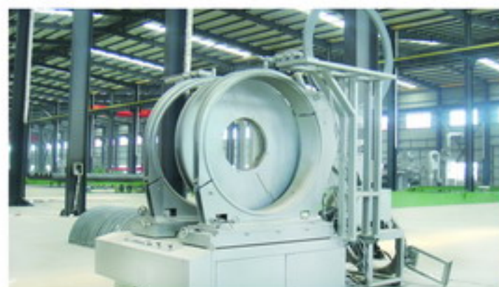
聚乙烯热板焊机 (RBH1600) polyethylene hot plate welding machine
