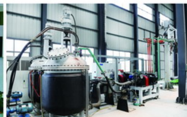
HPW350高压发泡机 HPW350 high-pressure foaming machine
