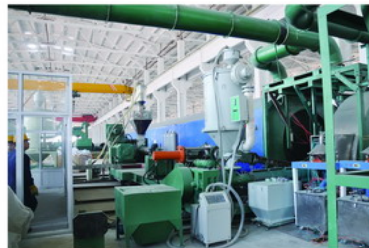
3PE (3PP) 防腐钢管PE,AD挤出机, FBE喷涂设备 Φ32mm-Φ1820mm PE, AD Extruder, FBE Spraying Equipments For 3PE (3PP) Coated Steel Pipes O.D.32mm-O.D.1820mm
