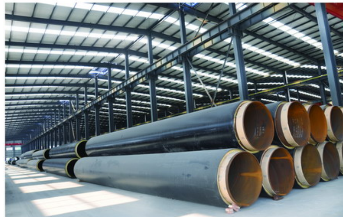
预制直埋保温管 prefabricated directly buried thermal insulation pipe
