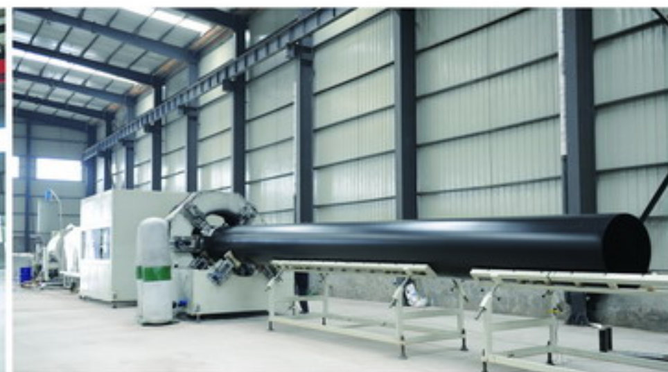
真空定径PE管生产线 (STV1800) vacuum sizing PE pipe production line
