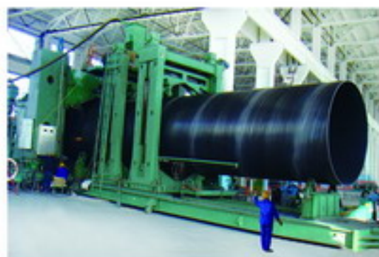
螺旋机组 \Phi 3620\text{mm} (局部) SSAW Pipe Production Line For O.D.3620mm (Part)
