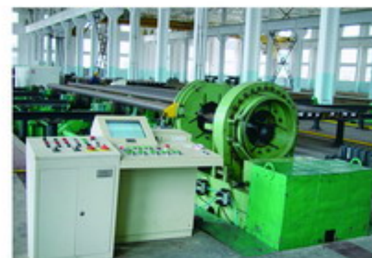
接箍拧接机 Screwing machine for coupling
