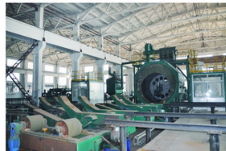
环氧防腐钢管内壁抛丸清理机 Φ508mm-Φ3620mm Internal Shot Blasting Cleaning Machine For Epoxy Coated Steel Pipes O.D.508mm-O.D.3620mm
