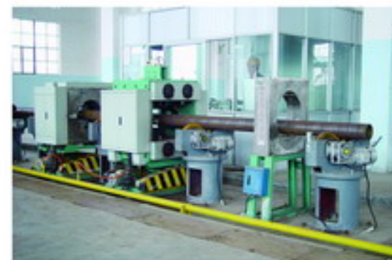
石油套管静水压试验机 Hydraulic pressure test machine for casing pipe
