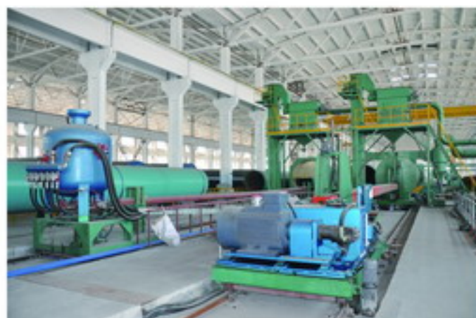
3PE (3PP) 防腐钢管内壁抛丸, 喷丸清理机 Φ32mm-Φ1820mm Internal Shot Blasting Cleaning Machine For 3PE (3PP) Coated Steel Pipes O.D.32mm-O.D.1820mm
