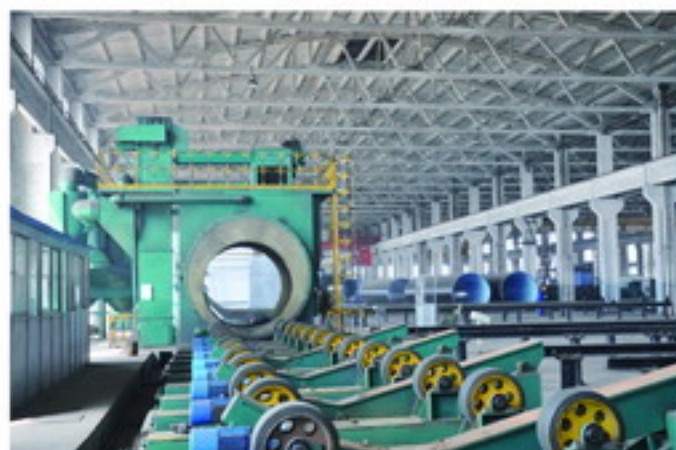
环氧防腐钢管外壁抛丸清理机 Φ508mm-Φ3620mm External Shot Blasting Cleaning Machine For Epoxy Coated Steel Pipes O.D.508mm-O.D.3620mm
