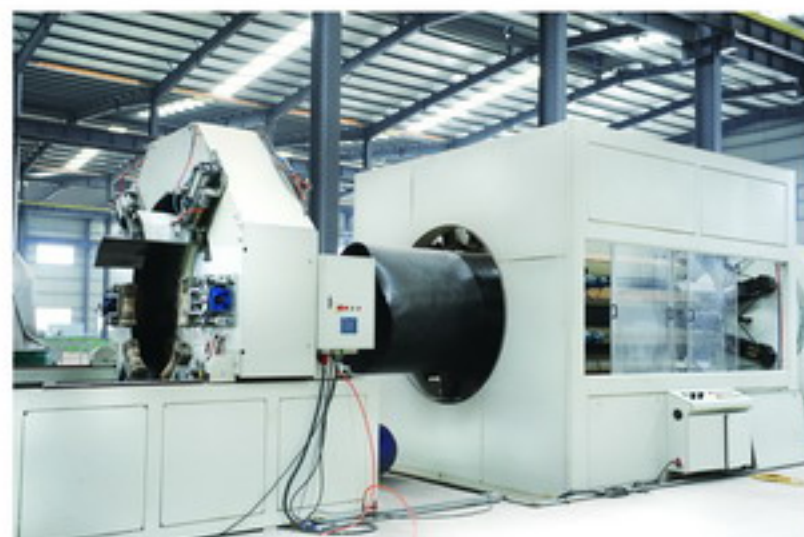
真空定径PE管生产线 (STV1800) vacuum sizing PE pipe production line
