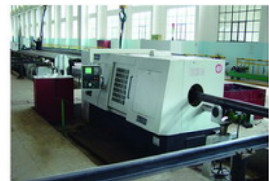
SUC0203 数控管螺纹车床 SUC0203 Numerical control thread cutting lathe
