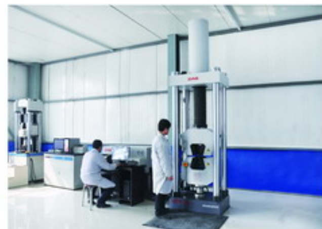
1000kN微机控电液伺服万能试验机 1000kN Electro-hydraulic Servo Universal Testing Machine
