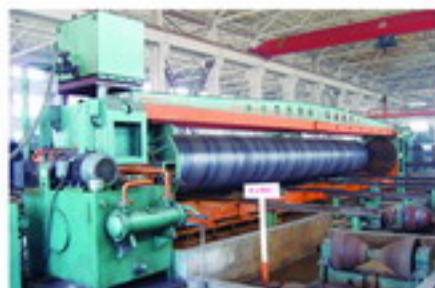
螺旋机组 \Phi 3620\text{mm} (局部) SSAW Pipe Production Line For O.D.3620mm (Part)
